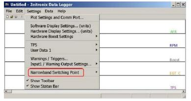
Open the Zeitronix Logging Software. Connect the Zt-2 Wideband AFR Meter into a PC COM port and power up the Zt-2. Make sure the log graphs are shown on the screen. Open the Narrowband Switching Point menu by selecting Settings/Narrowband Switching Point
