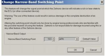
To Change the Narrowband Switching Point, adjust the number in the menu and click OK. The Narrowband Switching Point can be restored to a default value of 14.7 AFR by clicking on the Default Value, then OK.
